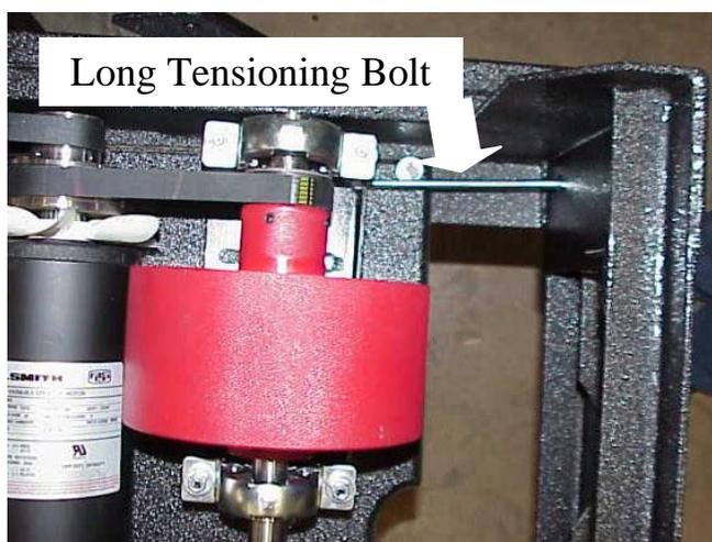
Use a ½” socket wrench to tighten the tensioning bolt just enough to remove the slipping. Check the tension on the belt that runs from the motor to the front roller by twisting or wiggling it.
