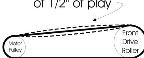
When the motor belt has the correct tension, tighten **only** the four bolts that hold the motor to the floor of the motor compartment. Do not tighten the bolts that hold the flywheel in place at this time.
